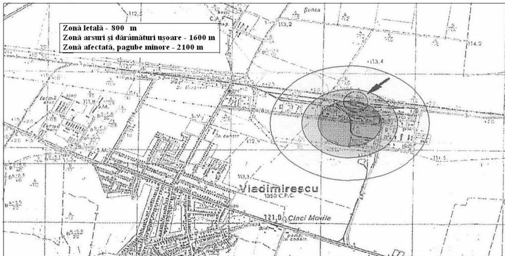
Fig. 1. Simulations with explosion scenarios
