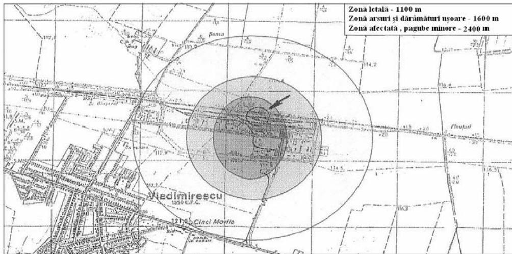
**Fig. 3.** Explosion risk in transporting LPG on pipelines, valves and pumps, which ensures the transport from rail ramp to the tank park and from the park to the technological loading line
