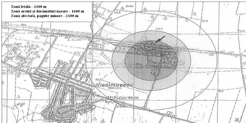
Fig. 2. Explosion risk in the technological process of bottling the cylinders
